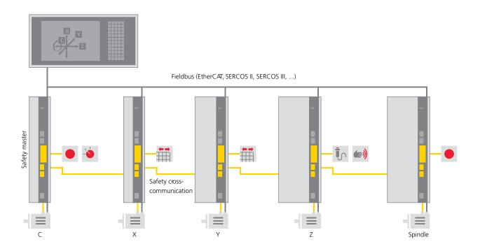
The safety control integrable into the ServoOne meets all your needs in terms of safe motion and communication:
